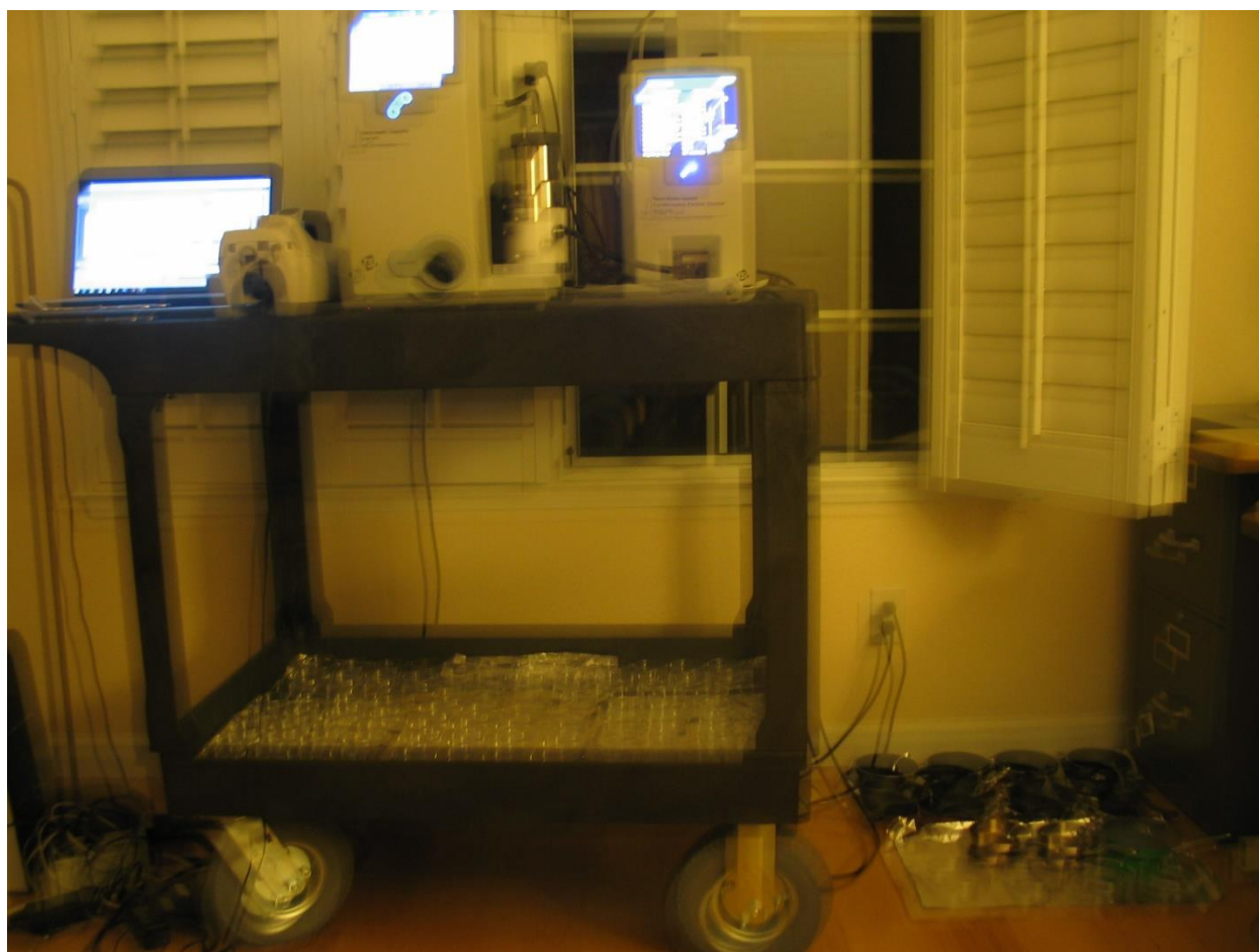
CPC, SMPS, and Petri dishes set out for exposure to SVOCs
