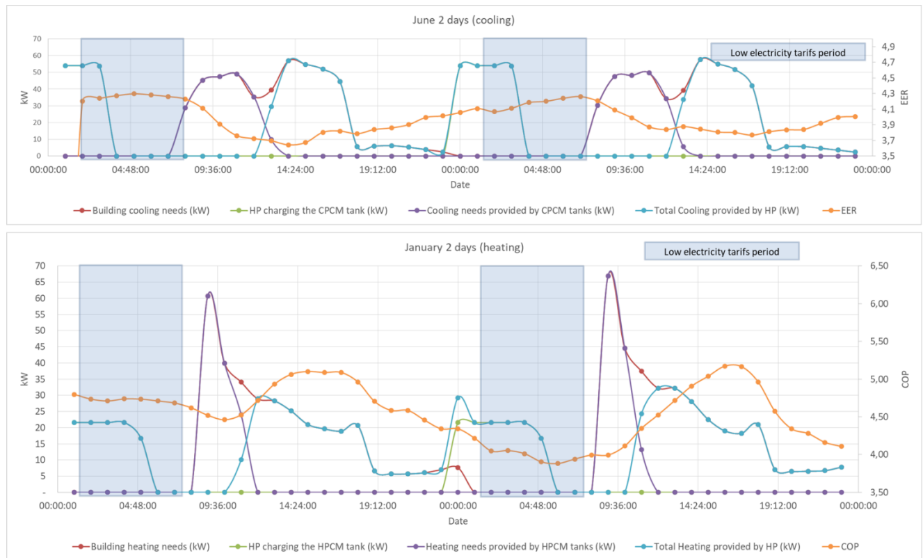
Figure 9 System operation for two typically days of cooling season and two typically days of heating season (Barcelona case)
