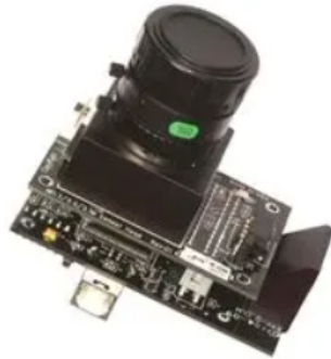
Figure 2.12: Aptina MT9P031 image sensor
