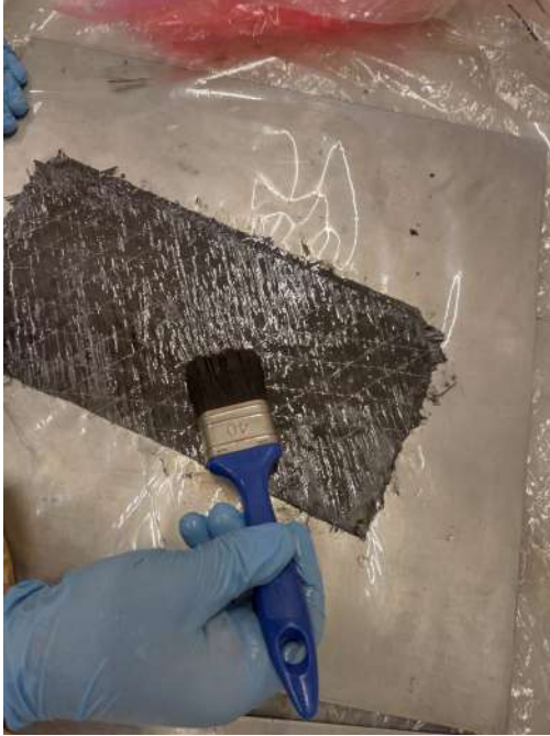
Figure 3.1: Wet hand layup process.
