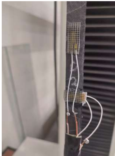
Figure 3.7: Specimen with strain gauge wired.
