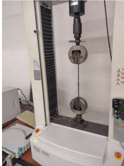
Figure 3.10: Tensile testing setup used.
