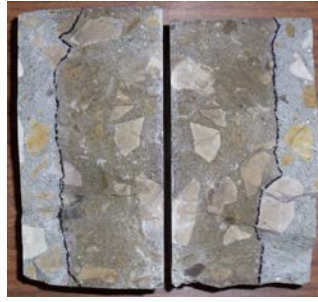
Figure 2 Slip open concrete specimen sprayed with \text{AgNO}_3
