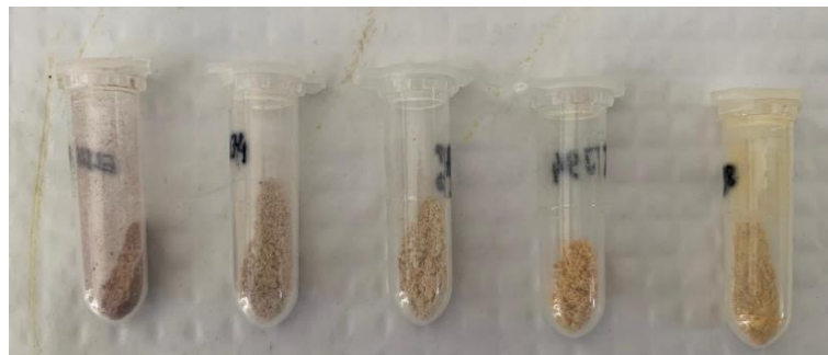
Figura 5.14 - Catalisadores ZnMOFs usados [\text{Zn}(\text{L}1)(\text{NMF})]_n , [\text{Zn}(\text{L}1)(\text{DMF})]_n , [\text{Zn}(\text{L}1)(4,4'\text{-Bipy})]_n , [\text{Zn}(\text{L}2)(\text{DMF})(\text{H}_2\text{O})_2]_n \cdot n(\text{H}_2\text{O}) , [\text{Zn}_2(\text{L}2)_2(\text{DMF})(\text{MeOH})]_n (da esquerda para a direita).
